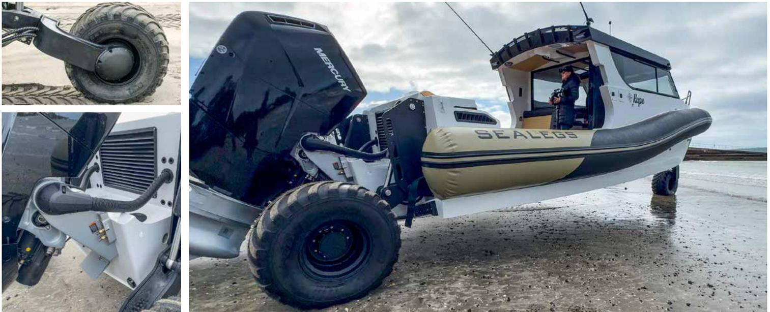
position. *Kupe* doesn't have a boarding ladder, so this ability to squat makes it easier to scramble on over the wheels at the transom, utilising the well-positioned hand-holds. (There is also an option of an electrically driven swim platform which extends out the side of the hull, but that box didn't get ticked, to save weight.) This 'squat' function also makes it easy to drain any water out of the bilge.
