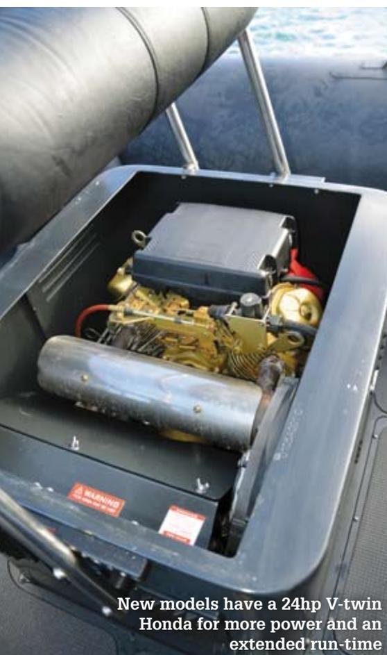
New models have a 24hp V-twin Honda for more power and an extended run-time
