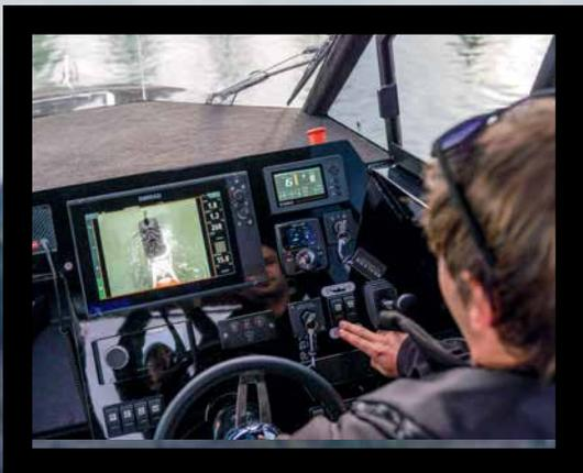
**INSET** the bow camera is aimed at the front wheel and the ground below it. It displays on the Simrad MFD.
